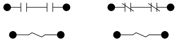
HXX (SPST N.O. Double Make) XXH (SPST N.C. - Double Break)
